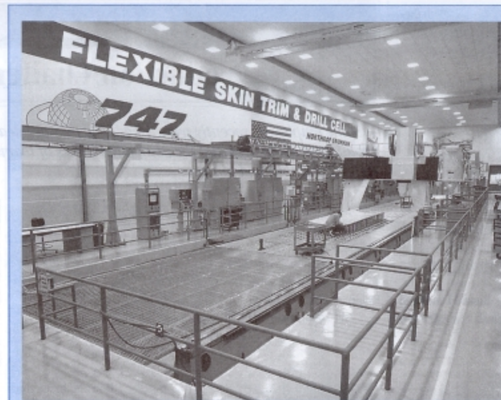
A Northrop Grumman employee checks a 747 panel section before it is trimmed and drilled by the company's new flexible skin trim and drill machine, also known as the "Pogo." These panel sections and others like it eventually will be assembled at Everett using new tooling designed by the Fuselage Assembly Improvement Team. Photo courtesy of Northrop Grumman.
